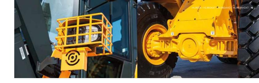
The **axles** of the HL960AHD are designed for uncompromising reliability during continuous heavy-duty work. Despite its great stability and power transmission capacity, the wheel loader axle has a compact design and low weight. The use of wet multi-disc brakes reduces braking losses and thus improves efficiency.
