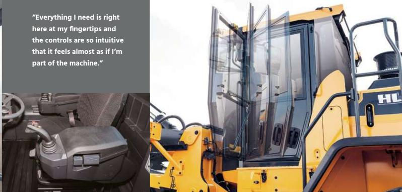
The HL960A has a large comfortable seat with heating as standard. The seat and armrest are fully adjustable and, for added comfort, an air suspension version is available as an option. Thanks to the electro-hydraulic implement control lever, less force is needed to operate attachments, helping you to work longer and more productively.
