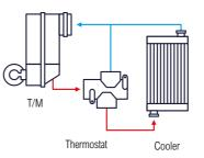
The HL960A is equipped with a **thermostat for transmission cooling**. This feature helps to warm up the fluid quickly and keeps it at the optimal working temperature, protecting components and increasing efficiency.
