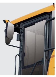
Foldable side mirror The side mirror is easy to adjust for optimal visibility and can be folded away to prevent damage during transportation.
