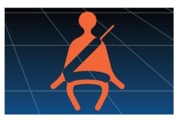
Seat belt warning alarm Operators are reminded to fasten their safety belt by an audible and visible alarm.
