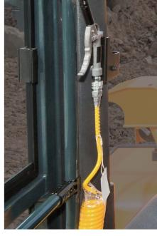
Air compressor An optional air compressor can be mounted in the cabin to help operators keep their workspace pleasant and comfortable.
