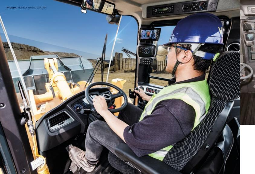
The HL980A has a **large**, **air suspended**, **comfortable seat** with heating as standard. The seat and armrest are fully adjustable.
