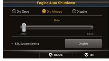
The engine shuts down automatically when the machine is at rest to cut fuel consumption and prevent unnecessary emissions. Different operating modes and idling times can be selected according
