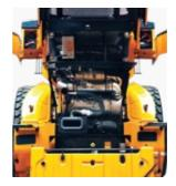
The engine hood is fully retractable and can be opened electrically for easy access to the sealed engine room and cooling room. The engine room is designed to prevent the possibility of fire caused by the inflow of foreign materials.
