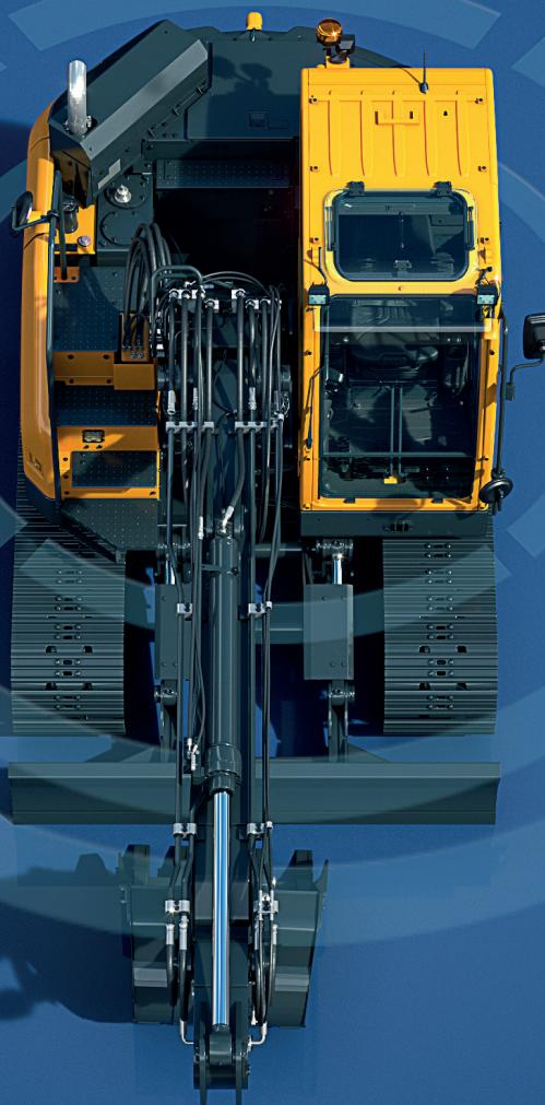
*Secure field of vision in all directions through ten views including 3D bird's eye view and 2D/4CH view.*
