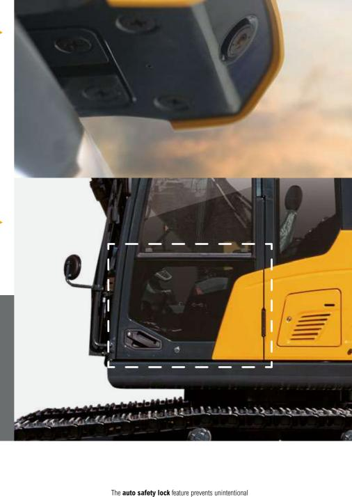
ignition. While the auto safety lock is activated, the excavator is not controlled by the RCV lever.
