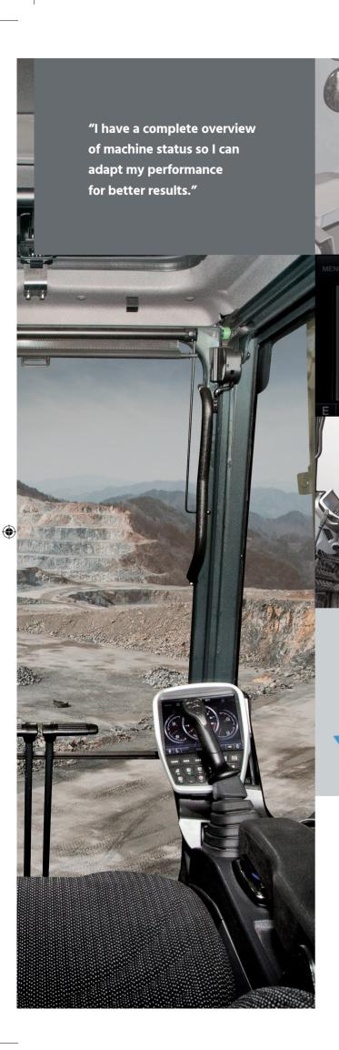
The instrument panel is optimised to provide quick, easy access to machine status information as you work. It features an 8-inch touchscreen monitor for excellent legibility.
