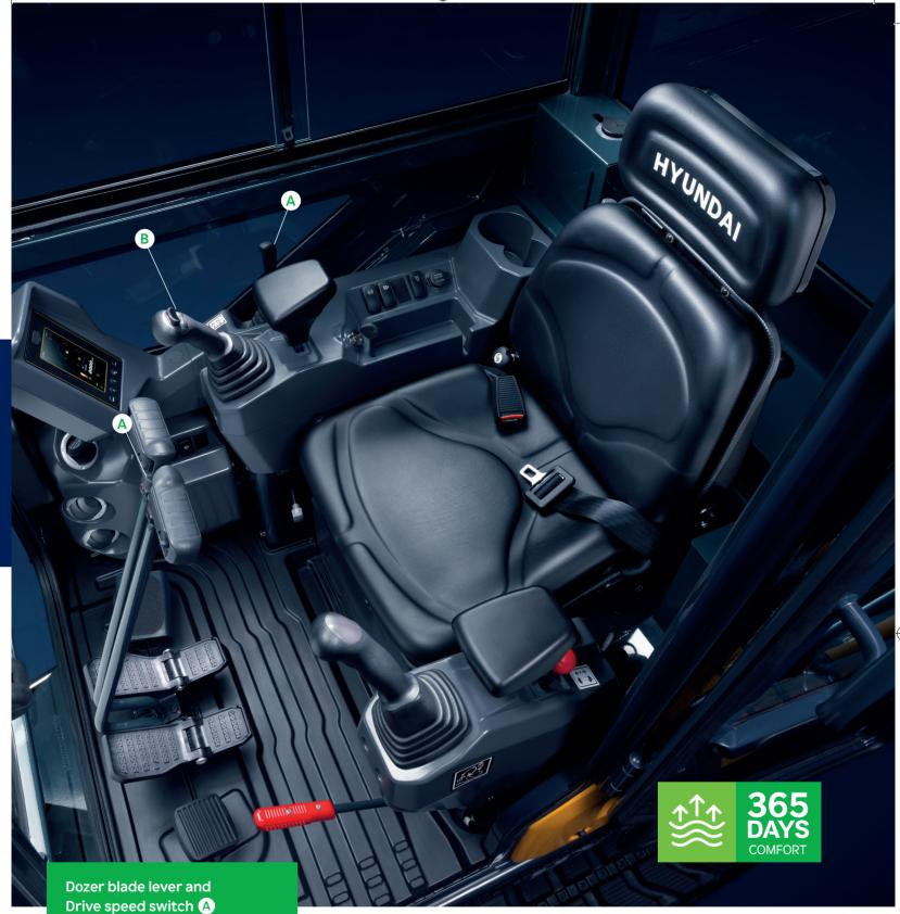
Two-handed operation for skilful and efficient levelling with drive mode changeover on the drive lever handle.
