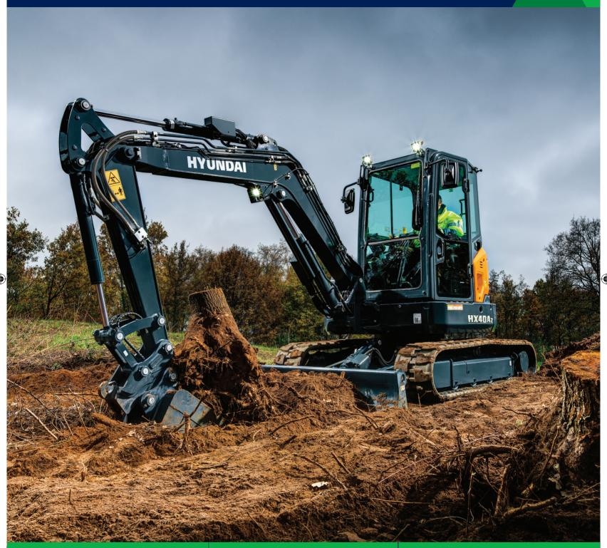
Engine Output 24.8 hp (18.5 kW) – 39.0 hp (29.1 kW) Bucket Capacity 0.11 - 0.15 m<sup>3</sup> Operating Weight 3880 - 5030 kg
