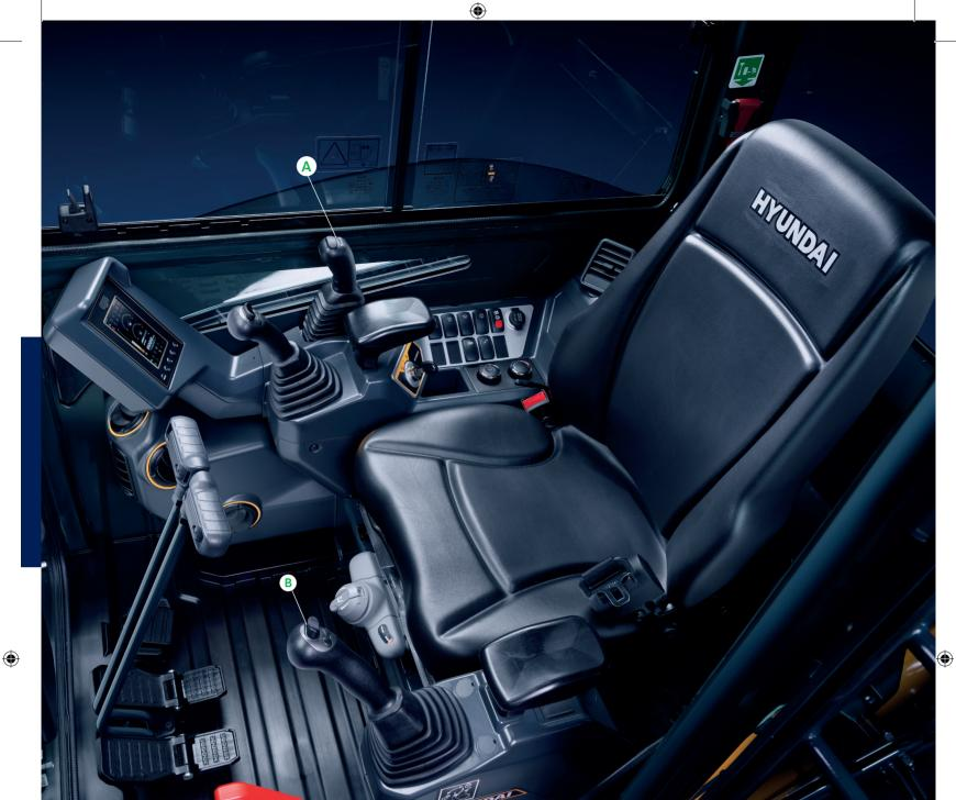
Use the dozer blade lever with fingertip control to define the perfect driving speed when grading.
